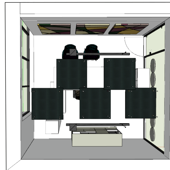
Room after acoustic adaptation - top view
